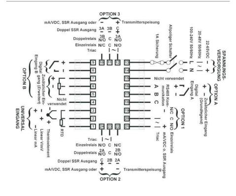
The wiring diagrams show all possible option combinations, whereby the necessary connections depend on the options fitted. Use single strand (max. 1,2 mm<sup>2</sup>) copper wire throughout, except for the thermocouple input, where the correct thermocouple or compensating cable and connectors should always be used.
